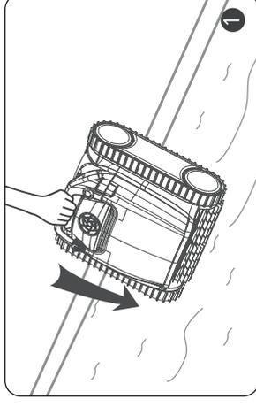
Hold the handle of the cleaner, and put it into the pool vertically.
