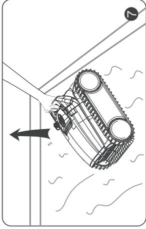
You should take the cleaner out vertically to drain inside water out quickly.
