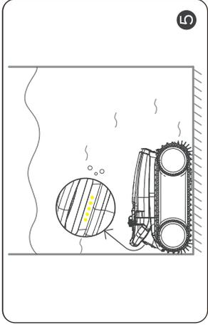
The device will automatically move to stop by the edge of wall when finishing cleaning or battery low.
