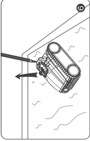
You can insert the included hook into a pool pole and lift the cleaner out of the pool.
